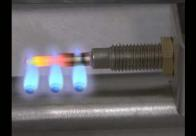
Dual Stainless Steel tubular burner bars run the full length of the roaster. Both are independently fed assuring total control of the cooking process and at all times
